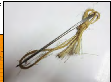
Vintage 6 inch sail needle made in Glyda, England used with baling twine to sew up used potato sacks filled with 50 lbs. of green cabbage.
