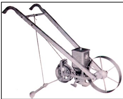
Many of the crops that required seeding in rows was accomplished by a Planet Jr. Hand-push Seeder.
